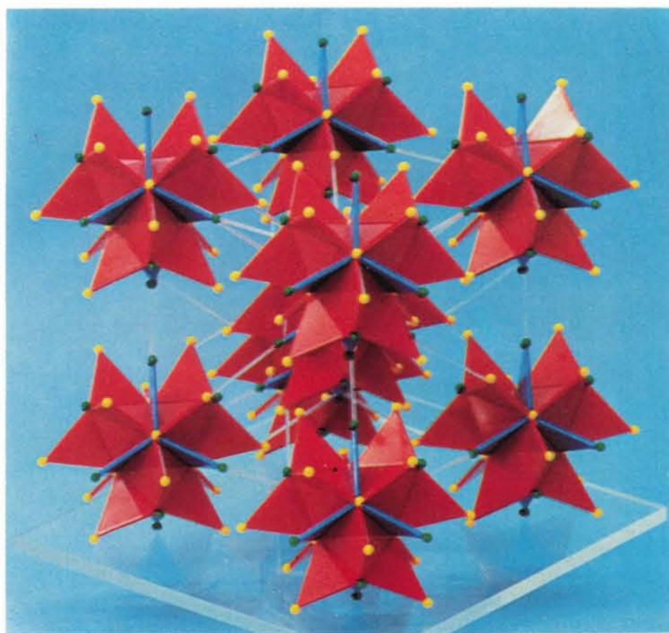
Fig. 6. Model of \gamma -brass. Green balls are Cu and yellow balls Zn atoms.
